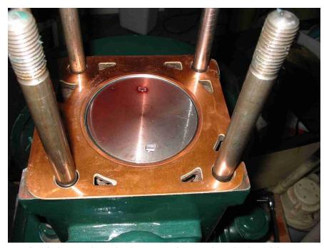
Indian head gaskets follow the design of the original Lister head gaskets. A copper fire ring is crimped over a copper/asbestos fiber/copper sandwich. The asbestos can be expected to wick coolant, so it should be sealed. I thought of using RTV silicone glue which is waterproof and resistant to heat up to several hundred degrees.
