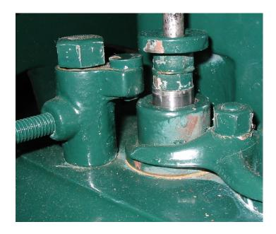
The decompressor arm which lifts the exhaust tappet seems to be a little short. It barely engages the flange on the lifter.
