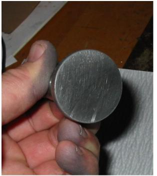
The cutter used to face the lifters appears to have been sharp. I saw no compelling reason to polish the surfaces further to a mirror finish, though I decided I'd lightly face them with 220 grit paper on a flat plate, then smooth the sanding marks on a buffing wheel with rouge.
