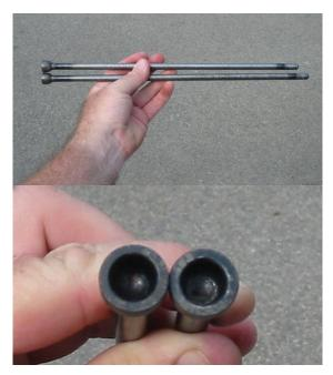
The pushrods were unpacked and cleaned of grease. The fact that both ends are hardened is evidenced by the discoloration that is visible at each end. The rods on the Ashwamegh were chrome plated. These rods will need to be painted before they begin to rust.
