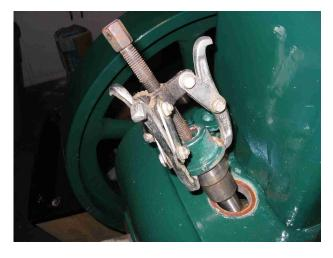
I ended up using a small 3-jaw gear puller to pull the intake guide past a rough spot of rust on the lifter stem. The lifters were then removed from inside the crankcase. The heat treated lifter faces are flat or slightly concave with concentric machining marks.
