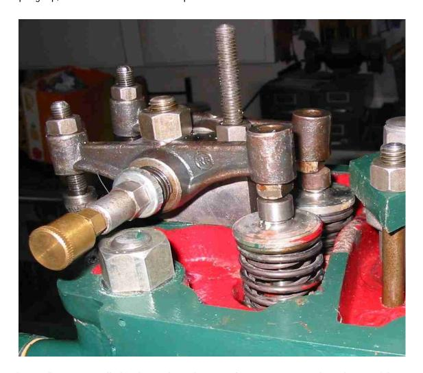
Some adjustment is called for here. The rocker arms don't register correctly on the top of the intake valve caps. That will place a small lateral force on the valve stems and wear against the cast iron valve guides.
