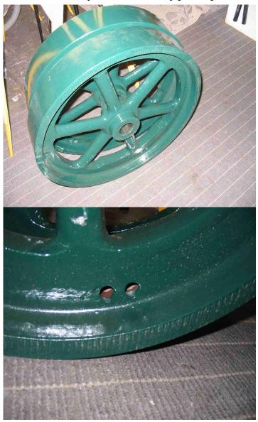
surprises in Indian castings without making more of them. If metal must be removed to achieve balance, and I don't believe that should be done, it should be removed from the web and not from the rim. A flywheel can more easily be balanced by adding lead weights to the rim without removing metal and weakening it.
