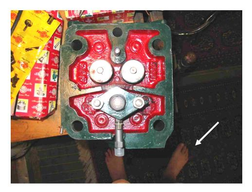
I replaced the valves, valve springs and keepers and installed the fuel injector. Again I have to say that the hardware that came with these parts was far superior to that on the Ashwamegh. Nuts, bolts and studs are thoroughly the equivalent of anything you'd find on an engine built in the West. And, yes, those are my bare size 13s. It's the middle of summer and I kept telling myself that I'd stop assembling after the next part and put some shoes on, but I was having too much fun.
