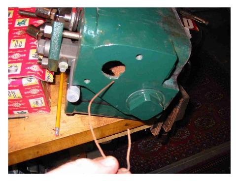
The water galleries in the head were free of casting flash and core sand, however I managed to remove a piece of bailing wire from the water outlet. The wire had probably been used to suspend the head casting from a hanger while it was being painted.
