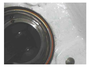
The cam lobes are located correctly to ensure tappet rotation. Note that the painter was careful to wipe paint from the machined surface above the TRB carrier at lower right. Note the tapered pin which holds the cam lobe on to the camshaft has been peened (sigh). If the hole was drilled correctly and assembled dry, the pin should hold without being peened as if it were a rivet.
