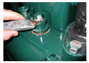
Vise-Grips on a part of the engine that will show, you can wrap a soft rag around the part to keep from scarring the paint.
