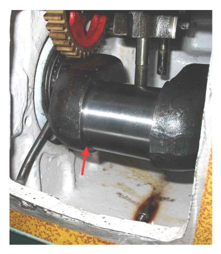
The pin appeared to have been carefully machined and polished to an appx. 400 grit finish. Low-level incident light indicated that the pin was cylindrical with no dips or grooves or visible machining marks and there was a generous fillet machined into each side of the pin. See red arrow in photograph. The importance of that fillet is discussed in the endnote. (2)
