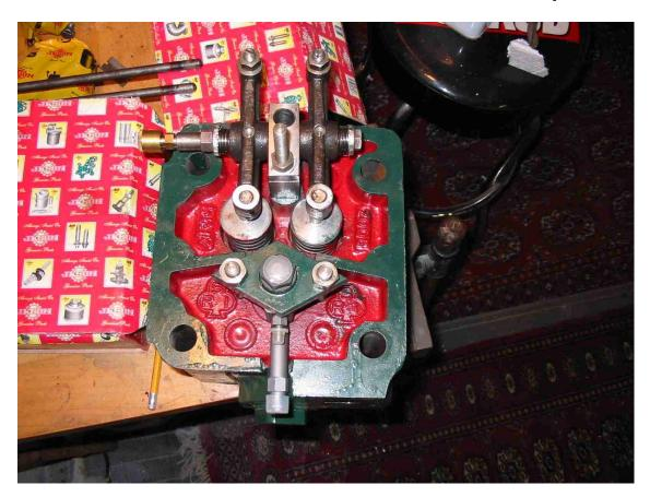
Below is a closeup of the rocker setup. Note the red and green paint on the valve springs and spring cap, which indicates the head was painted after it was assembled.
