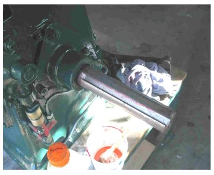
Acetone applied with a natural bristle paintbrush melted the red compound immediately but didn't affect the green paint. I was careful to keep the acetone away from the crankshaft oil seals.
