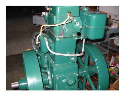
The fuel tank was installed and the fuel lines were connected. The fuel petcock was sealed with a piece of string which, like the head gasket, is an unnecessary throwback to the technology of an earlier day and doesn't instill confidence in the integrity of the valve. A quarter-inch ball valve adapted to the tank fitting with a quarter-inch British Standard Parallel Pipe Thread to NPT adapter, available from <a href="http://www.mcmaster.com">http://www.mcmaster.com</a> would fix that.
