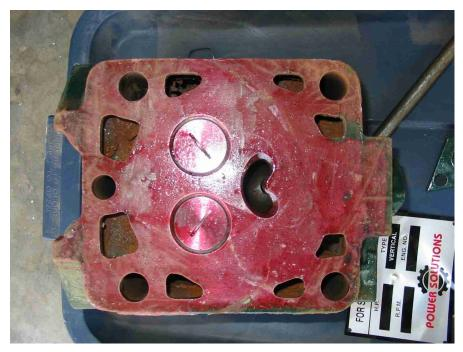
Once the anti-rust coating had been wiped off it was clear that the head had been nicely surfaced. The camera flash makes the surface dirt and rust in the water galleries appear much worse than it did visually.
