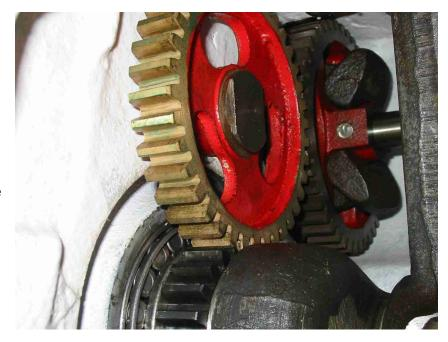
and ultimately broken timing gears.
