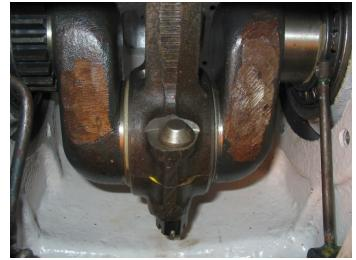
I knew the bearing cap nuts would be tight, the spec. calling for 50-60 ft-lbs., but it turned out they were *way* overtightened. I ended up needing to use an impact socket on a breaker bar with a 2' pipe slipped over the end to give me enough leverage to loosen the nuts. I was relieved when the nut loosened just as the wrench handle was approaching the side of the crankcase access hatchway. That's not usually my luck.
