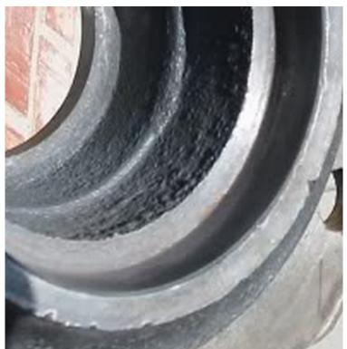
A close-up photograph shows the gritty surface. The grit was removed in a few minutes by using a wire wheel in the chuck of a portable drill. The surface is now ready for paint.
