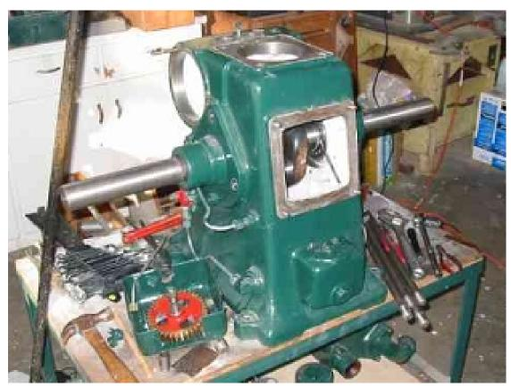
the crankshaft could not be turned by hand without exerting several ft-lbs of force which is a lot stiffer than I would have liked it to have been. It was clear that whoever assembled this engine wasn't very careful to avoid excessively pre-loading the TRBs.
