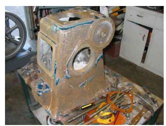
The next morning I lifted the crankcase out of the trash can and hosed it off. You can see in the picture at left that the paint removal was not 100 percent effective after only 8 hours soaking. I was too eager to see results and the concentration of drain cleaner wasn't enough to do the job in the time I allowed. There are still a few places where the paint didn't quite come off. And two areas in the bottom of the crankcase held bubbles of air, keeping the caustic
