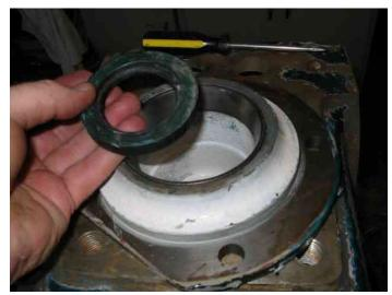
Gentle tapping on the handle of the screwdriver freed the seal without damaging it.
