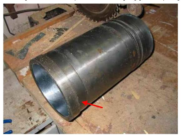
one on the cylinder casting which holds the cylinder liner in place. Rubber o-rings at the base of the liner prevent coolant from contaminating the crankcase.
