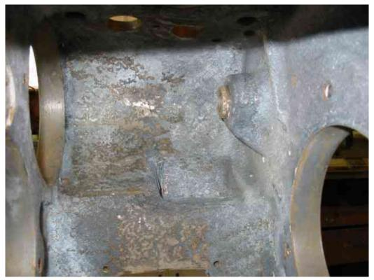
effectively sealed under a layer of paint. Unlike a gasoline engine, diesel engine crankcases are not a hostile environment to oil based enamel paints. There's no reason to use expensive two-part epoxy paints inside a crankcase. I planned to use the rest of the can of red Rustoleum enamel in a quart can that I painted the inside of my Ashwamegh with.
