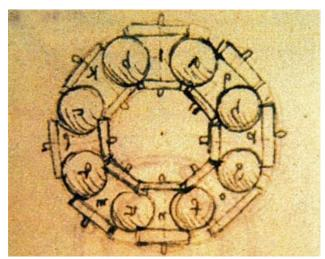
helicopter. That's right, a helicopter. This is the first recorded use of ball bearings in a machine. (2)
