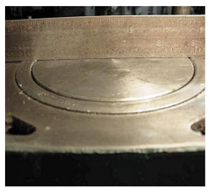
I balanced a straightedge on the top of the piston. I slowly rotated the crankshaft until the piston receded inside the cylinder, leaving the straightedge balanced on the liner with a sliver of light gleaming between the piston top and the bottom of the straightedge. The sliver of light was even, side to side. Had the piston been out of square with the cylinder casting, by even a couple of thousandths, it would have been visible. And if
