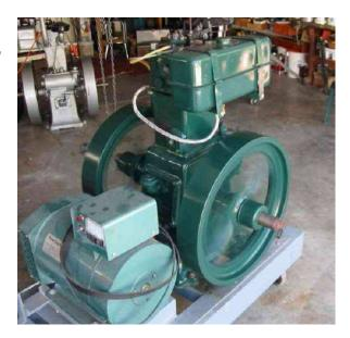
The engine settled down to a smooth and steady beat. No different in action or sound from my Ashwamegh. Tappets rotate about ½ turn each time they lift, the governor seems to be working well, and there are no fuel leaks. Even the petcock on the bottom of the tank does not leak a drop. And the engine seemed to be well balanced. My Ashwamegh is a very smooth running engine, and this one is no rougher, and possibly a little smoother.
