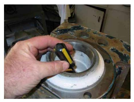
Before stripping the paint, I tapped out the TRB races and oil seals using tools I'm not proud of, and which I don't recommend: a screwdriver and a hammer. I know there's a better tool for this, but I don't have one. So I wrapped some cloth around the tip of the screwdriver and tapped gently.
