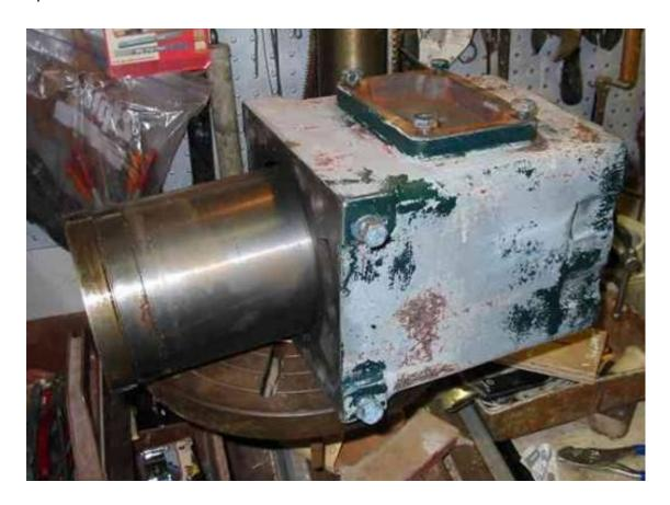
Note the location of the double grooves near the bottom of the sleeve for the O-rings and the ledge machined near the top of the sleeve. The ledge engages a corresponding
