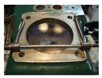
I removed the oil pump and oil lines from the crankcase. The oil distribution system has a crossover tube that lies just inside the big crankcase access door. While I was disassembling the engine in preparation to strip the paint, I puzzled for a while at how the crossover tubing could be disconnected. It appeared that there
