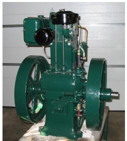
The British built Lister engines have attracted a loyal following by virtue of their excellence in design and quality of construction. Parts were carefully made from appropriate materials by skilled foundrymen and machinists. They were installed and fitted with care, and the result was an engine that was reliable ran for a long time with little maintenance.
