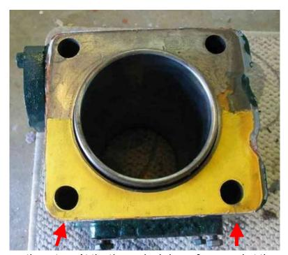
What the heck could that be? One 0.0075" thick half gasket had been stacked as a shim on the starting-flywheel side. Note the tears in the shim for the stud holes (red arrows). That indicates the shims were placed beneath the cylinder *after* the cylinder had been placed on the crankcase. I had been alerted to the existence of the yellow half-shims by Jack Belk, and John Ferguson emailed me that he had
