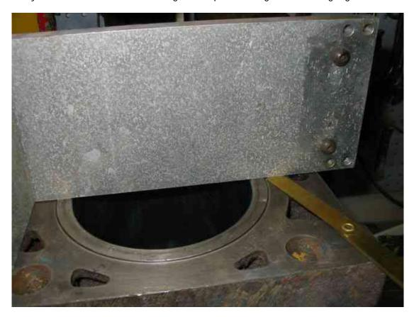
This measurement reveals two things. First, it indicates how square the sleeve is to the cylinder casting. Second, it will also indicate where there is excessive protrusion of the sleeve over the cylinder casting.
