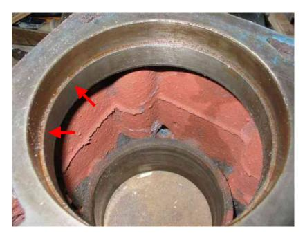
Looking down the bore of the cylinder casting in the picture below you can see a ledge (red arrows) machined into the cylinder casting that engages another ledge (red arrow in picture above) that projects out from the sides of the sleeve. These ledges must be clean (which they're not in the picture) or the cylinder will not be square to the casting
