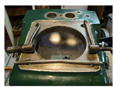
Here's a shortcut taken that nobody is likely to find until they tear an engine apart. Both ends of the crossover tube were ground to a taper but were never soldered. No compression fittings, no tapered seats. One wonders how much oil delivered by the pump leaked out of these fittings. It is fortunate that this engine is splash lubricated and that the oil pump is really not necessary for effective lubrication of the TRBs.
